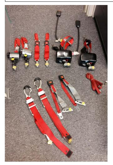
These are the wheelchair restraints and webbing straps which should be in this vehicle.
