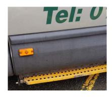
PASSENGER SIDE STEP. This is a large automatic step which is controlled from inside the vehicle – see below.
