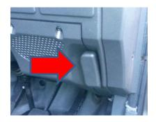
BONNET RELEASE LEVER: inside driver door, on right above accelerator pedal.
