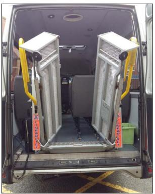
Use the control, found in a cradle on the left hand side of the lift, to deploy / stow the lift.
