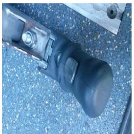
Seat release mechanism. Press silver button in and pull the lever back all the way. Tip seat forward to remove. To replace seat make sure lever is fully back, front legs are lined up in tracking and place back end in, push lever forward. Test seat is secure by shaking it strongly.
