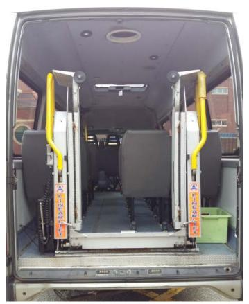
PN07 has the ONLY INBOARD TAIL LIFT in our fleet – it is also a split lift.
