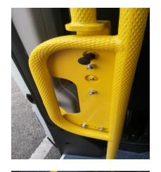
PASSENGER SAFETY HANDLES – release lever. There are two at the side door. Pull black button out making sure you hold on with other hand to lower down. To stow it, pull black button out again.
