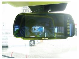
REVERSING CAMERA MONITOR: will activate when reverse gear selected. At all other times this functions as your internal mirror.
