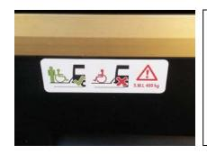
The maximum weight the tail lift can handle is 400 Kgs (62 Stone). That is the <u>combined</u> weight of the person(s) and the chair. Be aware of this max weight limit if a Carer is trying to get on the lift too.
