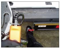
With the isolation switch on, use your foot to lift up the red handle on the side of the lift. Keep this raised while you activate the control stalk...
