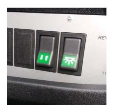
TAIL LIFT: In order for the tail lift to work, this isolator must be switched on (down). In this picture it is off.
