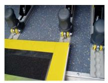
If you are using the tail lift solely to board a passenger who can walk and not using it to load a wheelchair: you will need to move the centre rear seat forwards to accommodate the large bridging plate.
