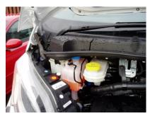
All the tanks to check. In the far left hand corner you can just see a purple cap cover, this is the screen-wash reservoir. Coolant, then brake fluid.
