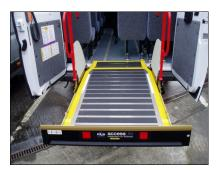
...with your foot still lifting up the red handle, press the up button on the control stalk. As soon as the lift starts to deploy, move your foot out of harms' way.
