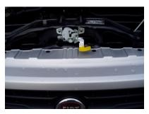
Position of the bonnet release catch, it's inline with the Fiat badge. Lift lever and pull bonnet up, secure it with the handle on right hand side.
