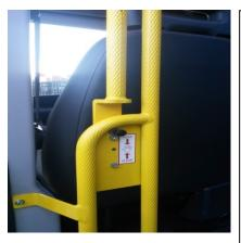
Passenger Handle release lever, pull black button out making sure you hold onto the yellow handle with other hand lower down and lock in, pull black button out to put yellow handle away.
