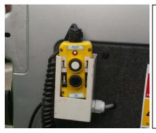
Tail Lift control, press the white Up/Out button to deploy the tail lift. Keep pressing up button until lift at the top, unfold lift as per instructions. To put lift away bring lift to top position and fold away. Press and hold the black Down/In to stow.
