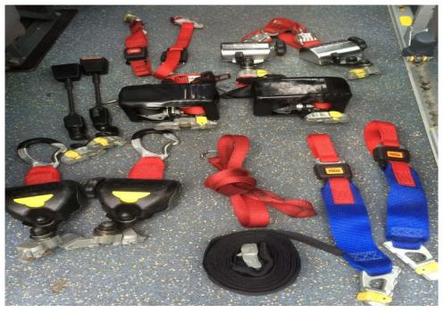
These are all the wheelchair restraints and webbing equipment which should be on FJ10RZN. They are stored in the box at the rear off side of the passenger saloon.
