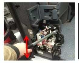
What to do if the power fails to this tail lift. A manual pump for the mechanism.
