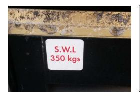
The maximum weight the tail lift can handle is 350 Kgs (55 Stone). That is the combined weight of the person and the chair. Be aware of this if a Carer is trying to get on the lift too.
