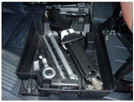
TYRES: This jack is under the front passenger seat and is removed by twisting the small, circular catch at the front left.
