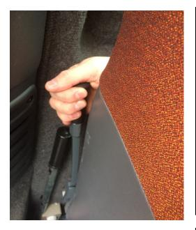
Get a good hold on the handle as shown and pull firmly towards the front of the bus.
