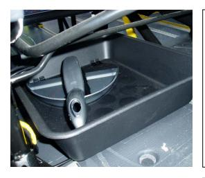
CLEANING: you can use this brush to sweep off the seats, tracking and floor. This picture shows a storage tray underneath the driver seat.
