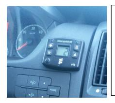
CAB HEATER SWITCH: press wavy lines button to turn on heat and fan symbol for "ventilation". Press a second time to turn off. Arrow keys up or down to desired temperature. Switch heater off at end of trip, day and when fuelling.
